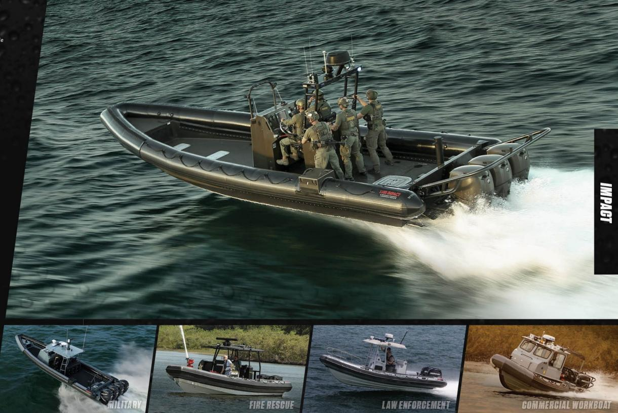
The Impact D features a hybrid air/foamfilled collar mounted to a solid fiberglass gunnel. Instead of a fully circular tube, our Impact D-collar allows for more space on deck and added maneuverability and versatility for the crew. The D-collar gives an RHIB. Law enforcement finds this design especially suited to tactical maneuvers, where boarding another craft may be necessary.
