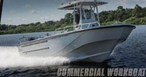
The Justice offers a deep-V hull and center console design making it well suited for offshore patrols. Whether navigating high-traffic areas or plowing through big waves, the Justice its higher free board and pronounced chine translating into a softer, drier ride.
