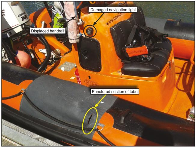
Figure 10: Damage to Osprey II
