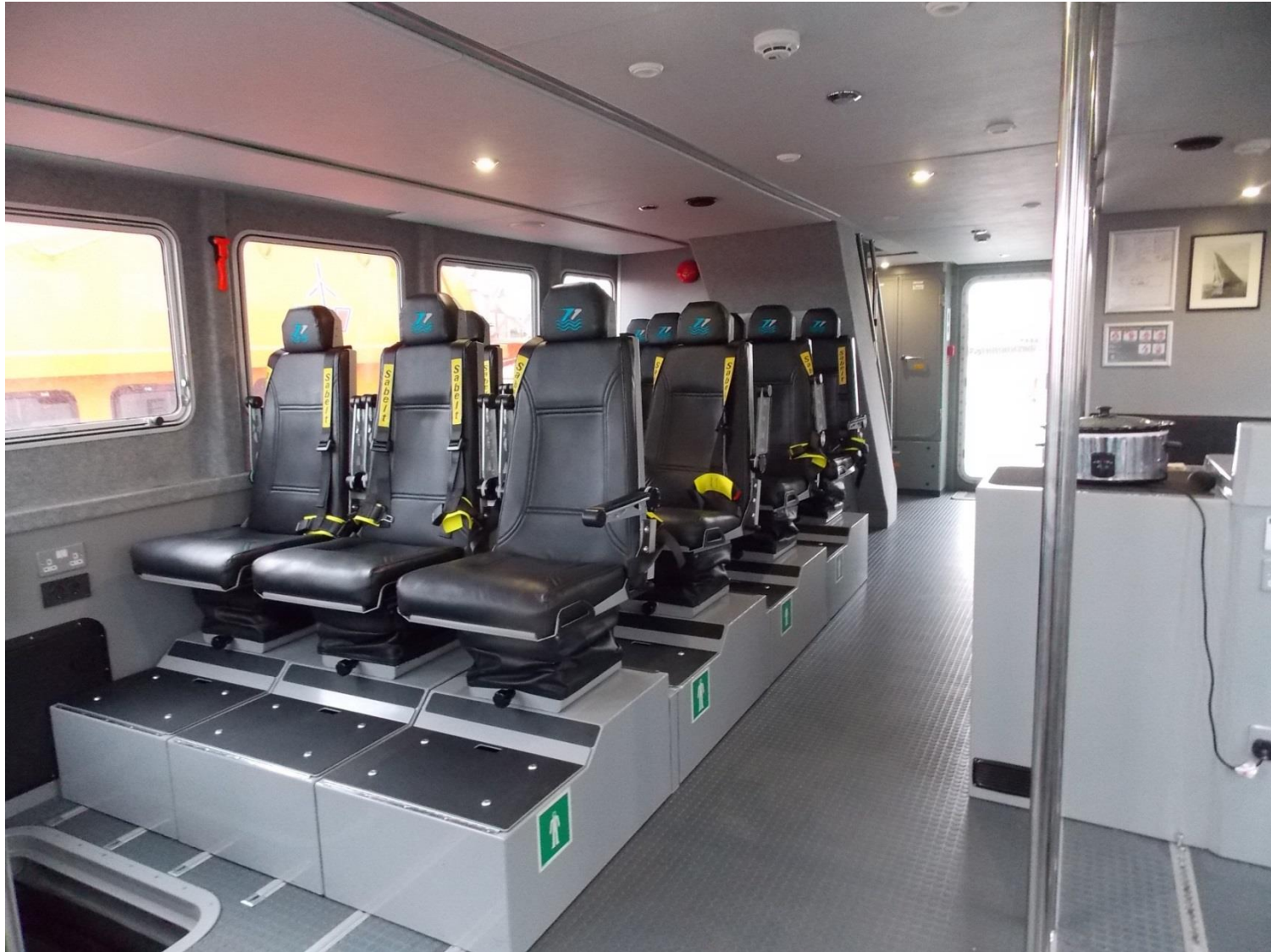
South Boats – KPM interior design after full design and crash test evaluation. Courtesy Sea Cat Services
