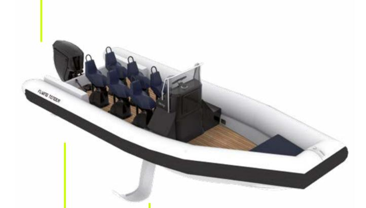
Electrically assisted retractable foils with simple push button activation for easy marina access, beaching and trailer transport
