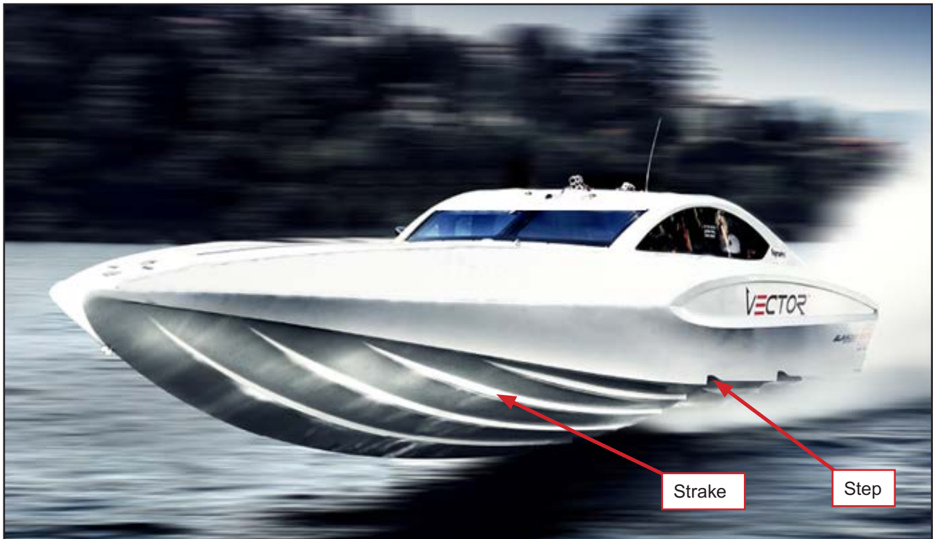
Figure 1: Stepped hull with multiple strakes
