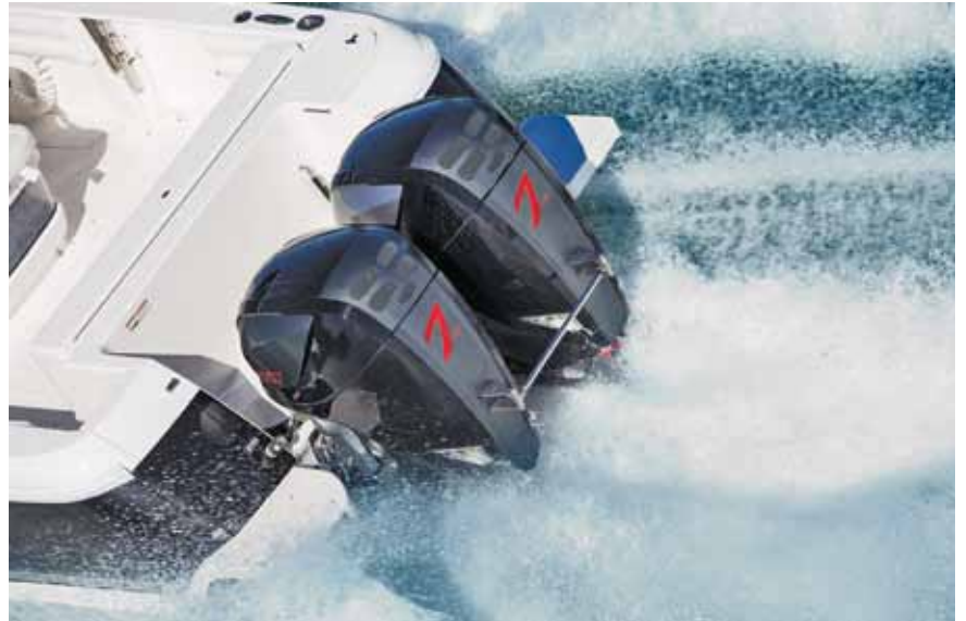
Twin Seven Marine 557 outboards: the newly launched, 415kW outboard was designed to grant small vessel users the same power with a two-engine arrangement as is typically possible with a four-engine set-up (credit: Seven Marine)
