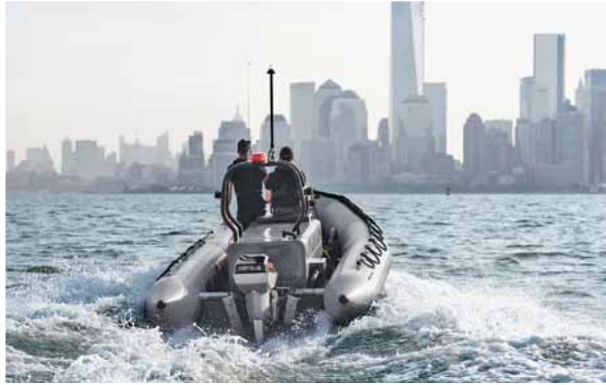
Torqeedo's battery-powered Deep Blue drive (left) comes in 30kW and 60kW single versions; the 60kW version has been deployed on Zodiac Milpro's SRM600 range of RIBs (right)
