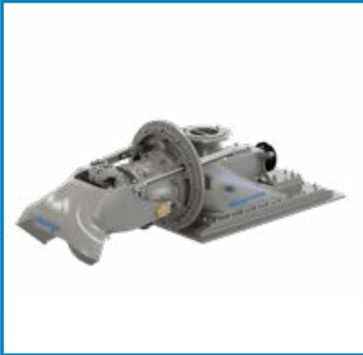
MJP Ultrajet Series are rated for commercial and military operating conditions. The Ultrajet Series feature a single-stage high-efficiency axial-flow pump with a variety of options to suit the vessel design and mission. A wide range of impellers match most marine diesel engines from 100 to 1340 kW (134 to 2172 hp) per jet with the appropriate direct drive or reduction gear ratio.
