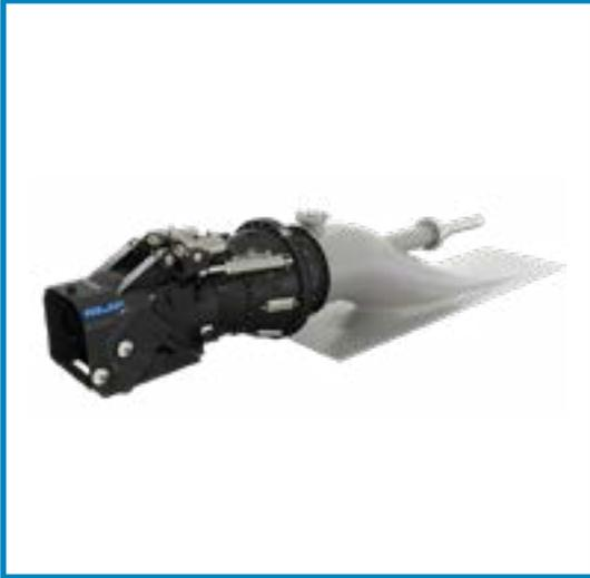
The Compact Steering Unit (CSU) is a well-proven mixed-flow all duplex stainless steel waterjet. Featuring a classic design with superior performance and long service life, the CSU is well suited for military and government applications, large commercial craft and passenger ferries. Power options are 2500 kW, 3000 kW, 4000 kW, 6000 kW. The MJP Electronic Control System offers complete control of the jet position and engine RPM control, thereby controlling all vessel motions.
